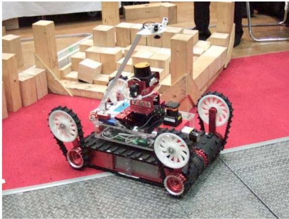
**Figure 1. 6-crawler mobile robot Kenaf**
